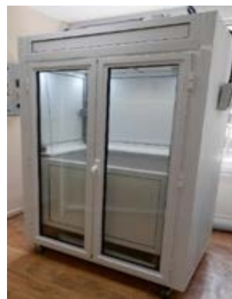
Fig. 2. Thermal insulated chamber The average and upper levels of the factor x_2 correspond to 50% of the field capacity (FC) and of the FC
