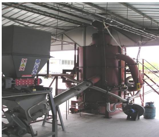
Fig.1 Realized installation for utilization of biodegradable waste, production of biochar for application in BioCCS practices
